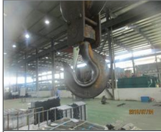
Photo of the inside of the main production hall Correction 7.17 Lock installed in travel cranes hook.JPG
